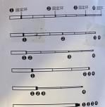
通过将相邻两个定位环的 结合实现不同长度的调节 Realize different length adjustments by combining two adjacent positioning rings.
