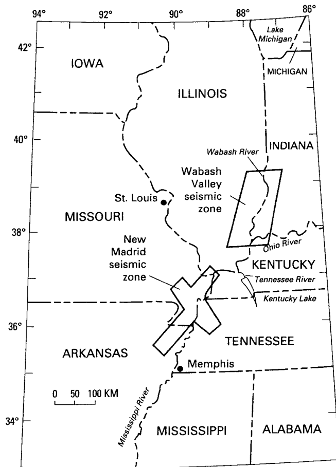
Figure 7.11 Approximate limits of New Madrid seismic zone and Wabash Valley seismic zone. New Madrid seismic zone is the source area of the 1811–12 earthquakes and continues to have many small earthquakes and a few slightly damaging earthquakes. The Wabash Valley seismic zone is a weakly defined zone of seismicity having infrequent small to slightly damaging earthquakes.
