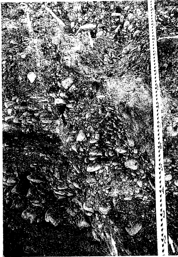
Figure 2.17 Close-up photograph of two parallel normal fault strands (between arrows) in gravelly late Pleistocene deltaic deposits, East Bear Lake fault, Utah. Numbers on rod are 10 cm apart. Note anomalous parallel clast fabric and slight discoloration of gravel along the fault strands.
