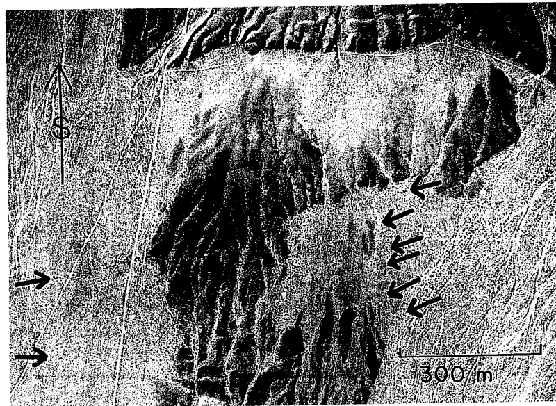
Figure 2.2 Vertical aerial photograph showing east-west-trending normal fault scarps (in shadow at top, and in center) and parallel lineaments (between arrows) that overlie buried faults. Ephemeral streams flow from top to bottom. Note dissection of scarp at top of photo and secondary alluvial deposition on the downthrown fault block at upper center. Lone Mountain fault zone, Nevada. (Photograph courtesy of J. C. Yount.)
