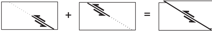
Figure 12.1. Steady slip below a locked seismogenic zone added to coseismic slip on the shallow fault leads to rigid body motion. Note that for dip-slip faults, the rigid body motion includes nonphysical vertical displacements of the earth far from the fault.
