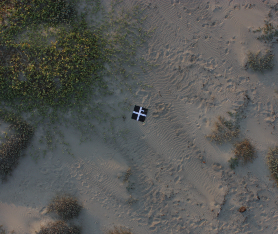
A ground control point marker. Image courtesy of Michele M. Tobias & Alex Mandel Creative Commons Attribution-ShareAlike 4.0 International CC BY-SA 4.0
