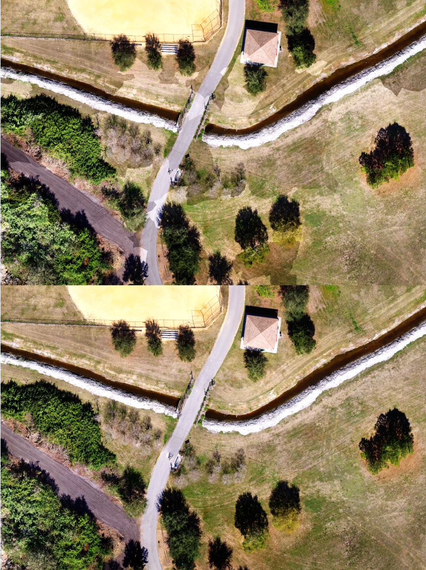
Seams in the textured model due to different illumination (top) and global seam leveling applied (bottom)
