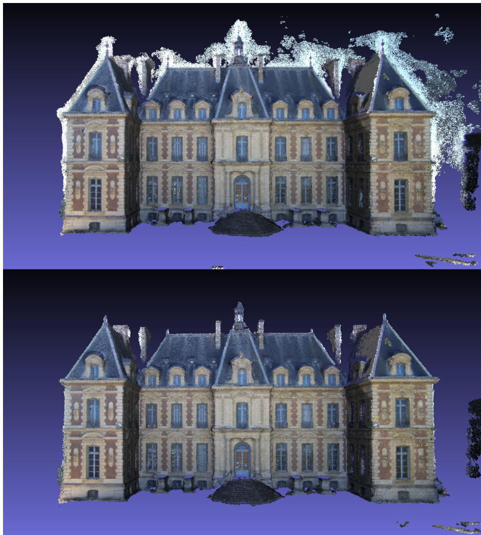
3D point cloud without (top) and with sky masks (bottom). Sceaux castle model generated from photos by Pierre Moulon 32
