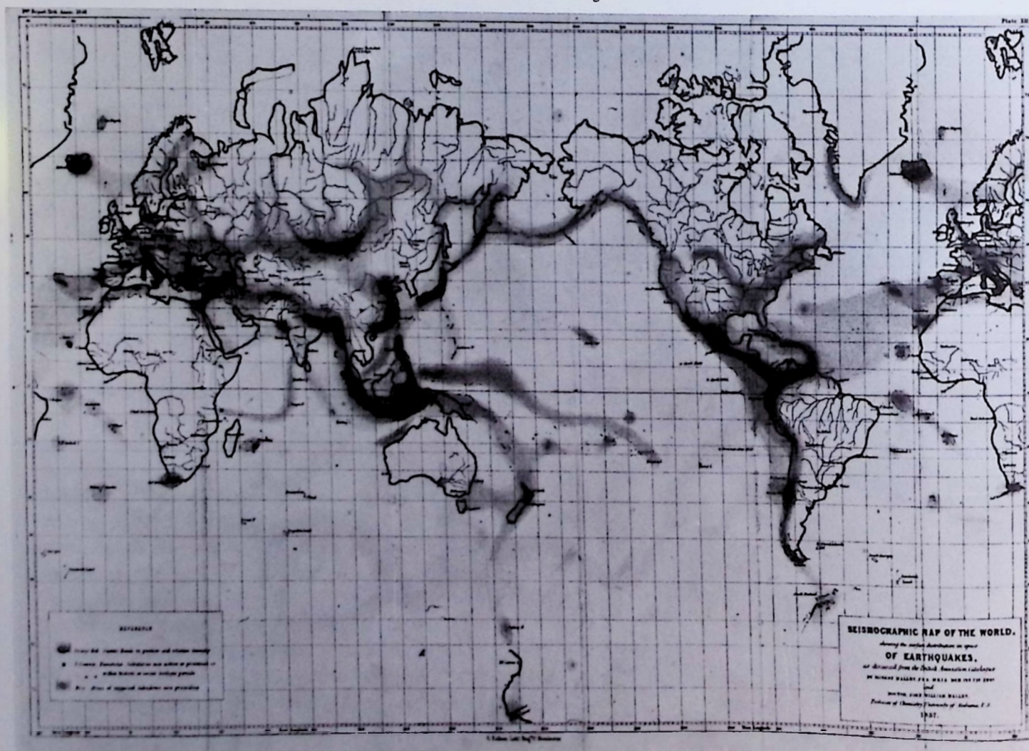
Figure 1. Map of the world showing the distribution of earthquakes, prepared by Robert Mallet on the basis of historical data and presented to the British Association in 1857 (28th Report of the British Association, 1858). Note the similarity of this map to the map of short-term, modern seismicity prepared on the basis of modern instrumental data shown in figure 2.
