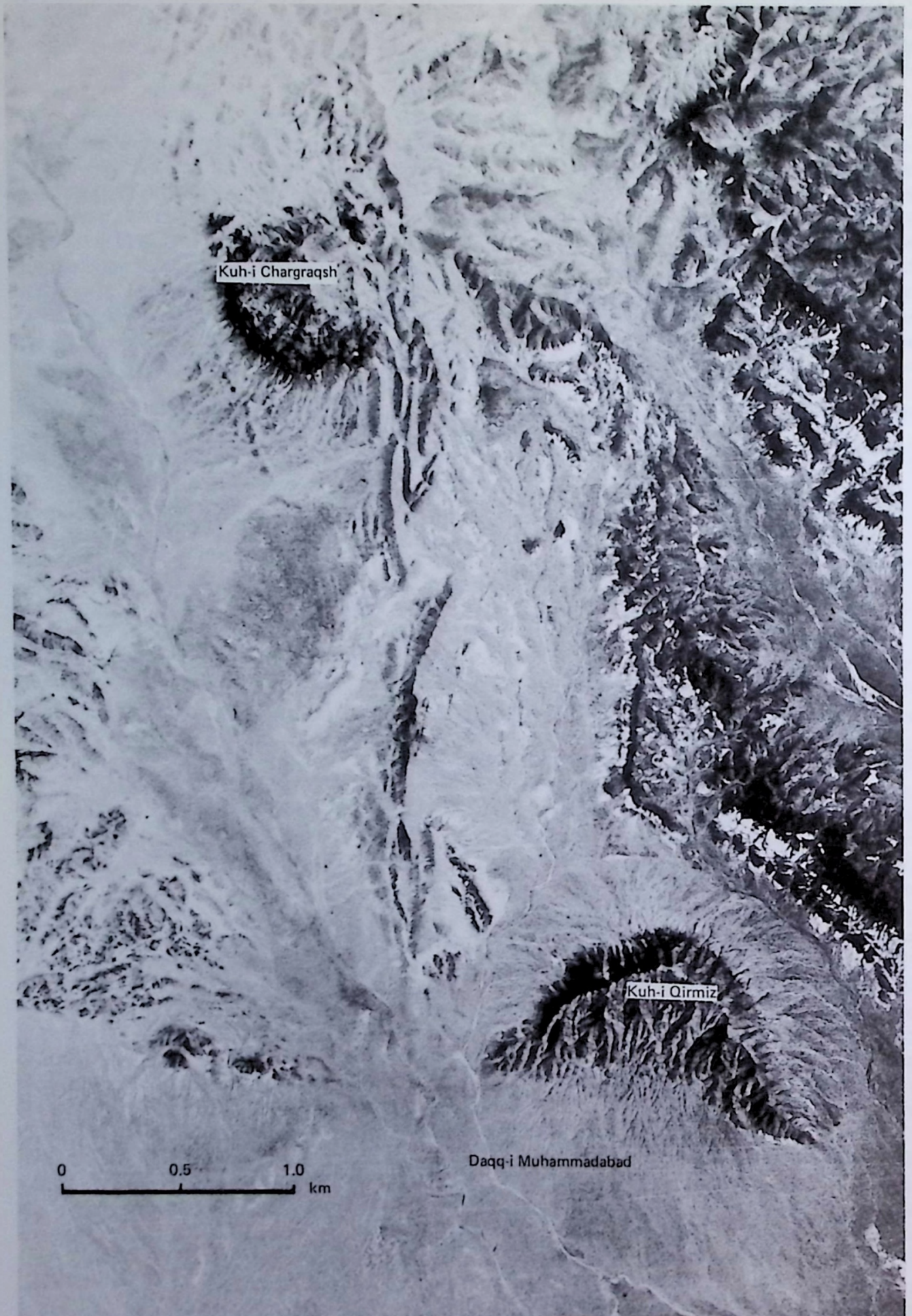
Plate 17. Aerial view of the Dustabad ground ruptures associated with the 1947 earthquake.
