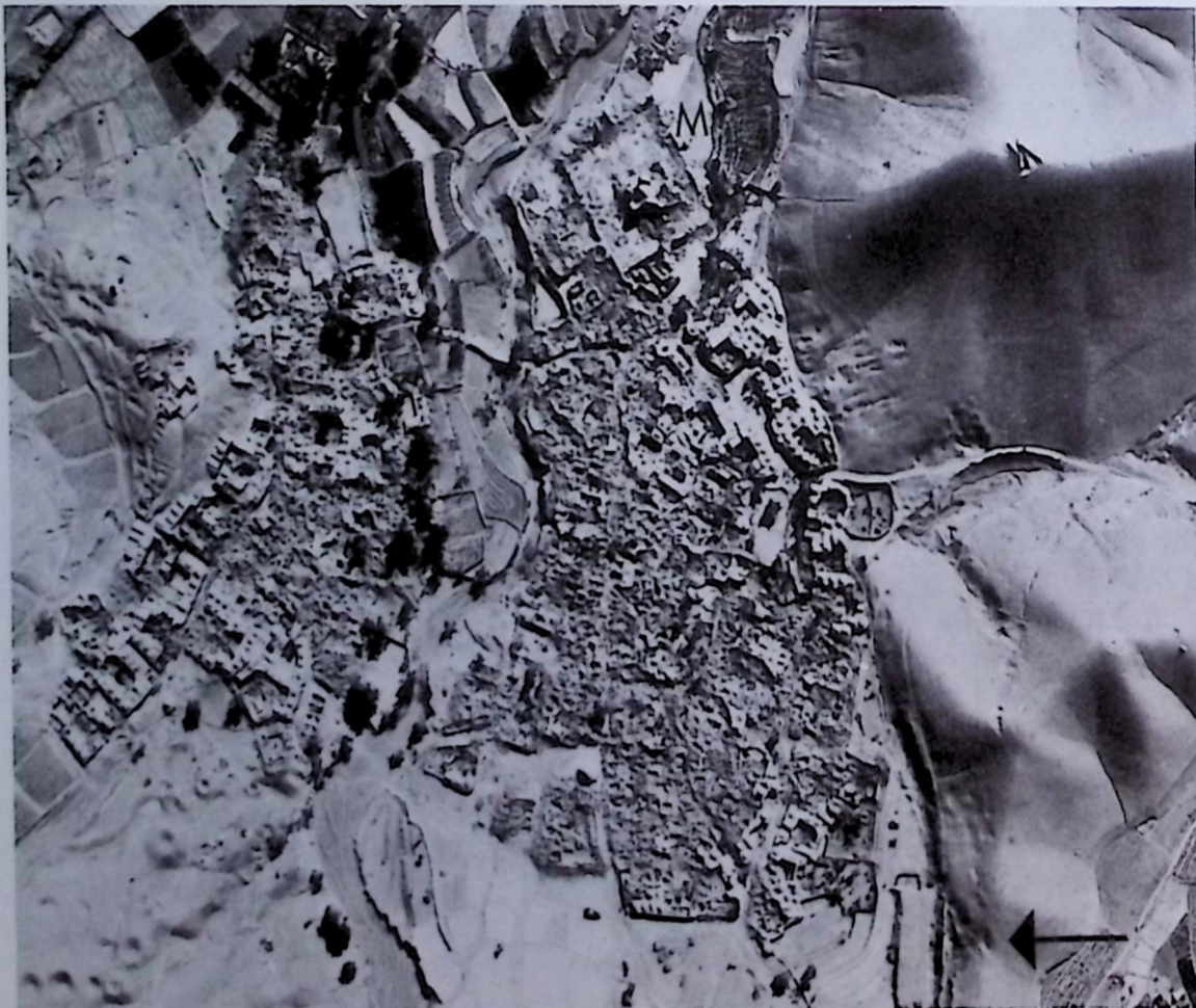
Plate 2(a). Damage to adobe houses built in clusters: Aerial view of the village of Kariskh (9 kilometres west of Dasht-i Biyaz) taken after the earthquake of 31 August 1968. Notice that with the exception of a few houses southwest of the mosque (M), the village was totally destroyed (80% of the houses collapsed killing 20% of the people, see Ambraseys & Tchalenko 1973).
