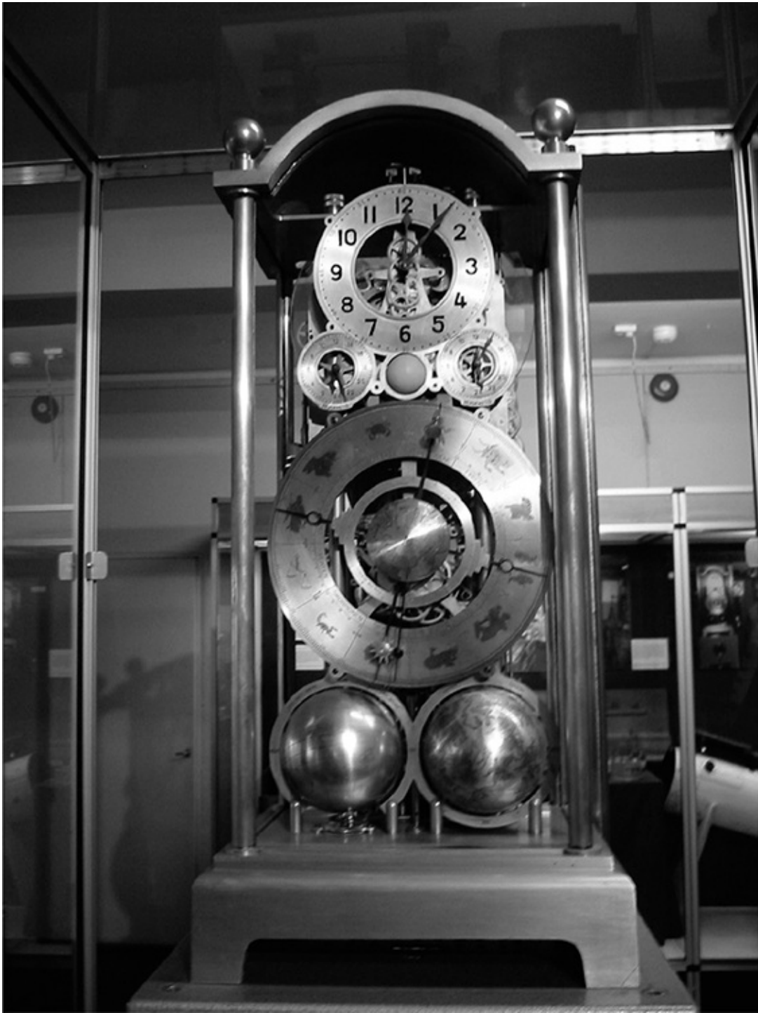
Astronomical clock (number 3) designed and made in Norway by Rasmus Sørnes. Finished in 1954, it computes a large number of time/astronomical values including sidereal time, sunsets and sunrises, Gregorian date, solar and
